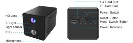
**How to reset camera:** Turn the power switch to "On", hold on the reset button for 5 seconds until you see the blue light and the green light turn on together, and then the blue light flashes slowly.
